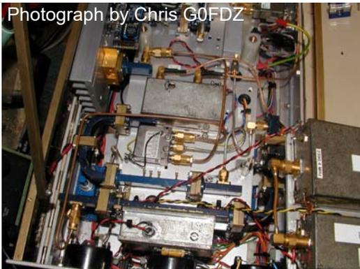
Modern Transverter system with a 2 watt HPA and GaAs FET LNA
